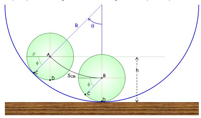
The CM moves along the arc,  $S_{CM}$  =  $(R - \rho)\theta$  and point C moves around the circumference of the sphere,  $S_C$  =  $2\pi\rho$ . This is a shorter distance than the arc length between the points of contact,  $S_{Bowl}$  =  $R\theta$ . This is because the contact point with the bowl changes even though the sphere has had a full rotation.
