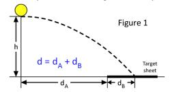
2. Your instructor will show you how to load and shoot the projectile. Measure the height, *h*, of the projectile above the floor (measure to the *bottom* of the picture of the projectile on the right side of the launcher). In your sketch, indicate the launcher you used (A, B, C, etc. – the label is on the vertical support)
