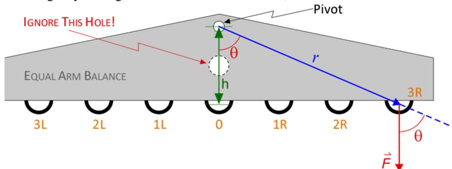
Figure 2: The Equal Arm Balance
