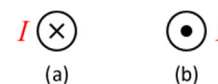
Figure 5: Showing direction of I (a) into the page and (b) out of the page
