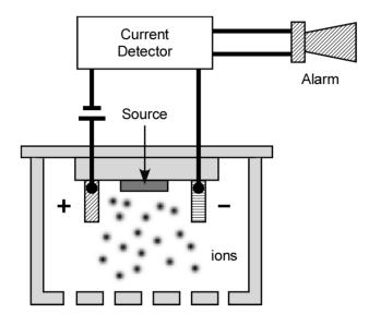
Appendix: How an Ionization-Type Smoke Detector Works<sup>1</sup>
