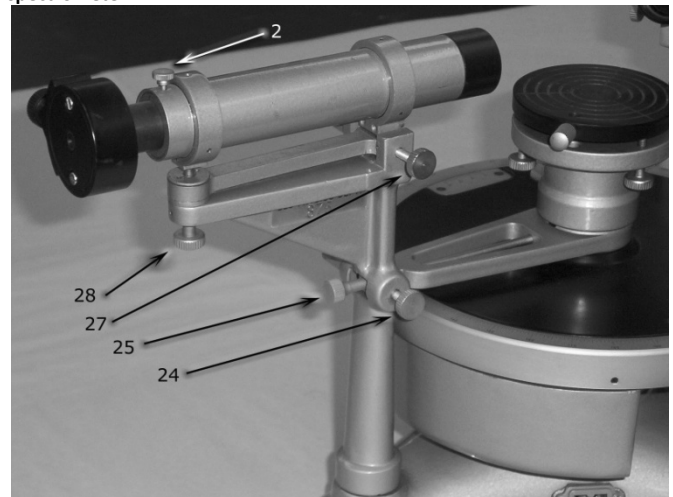
Figure 6 – Adjustments on the left side of the collimator
