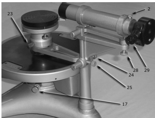
Figure 5 – Adjustments on the right side of the collimator
