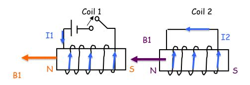
c) Since the switch is being opened, the flux is decreasing. TO oppose the change a current is induced in coil 2 that produces a B-field in the same direction as the field in coil 1
