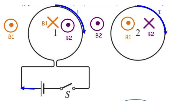
b) As the switch is closed, is the magnetic flux in loop 2 increasing, decreasing, or staying the same?
