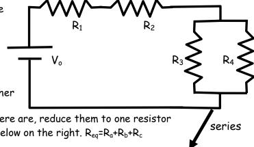
2. Look at the circuit and determine whether there are any resistors in parallel. If there are, reduce them to one resistor called  $R_{eq2}$ , and sketch the new circuit on  $1 \quad 1 \quad 1 \quad 1$
