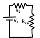
2. Look at the circuit and determine whether there are any resistors in series. If there are, reduce them to one resistor called  $R_{eq2}$ , and sketch the new circuit on the right.
