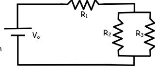
$$\begin{split} \frac{1}{R_{eqparallel}} &= \frac{1}{R_a} + \frac{1}{R_b} + \frac{1}{R_c} \\ &\frac{1}{R_{eq1}} = \frac{1}{R_3} + \frac{1}{R_2} = \frac{1}{R_3} \frac{R_2}{R_2} + \frac{1}{R_4} \frac{R_2}{R_2} = \frac{R_3 + R_2}{R_3 R_2} \\ &R_{eq1} = \frac{R_3 R_2}{R_3 + R_2} = \frac{40 \Omega \bullet 60 \Omega}{40 \Omega + 60 \Omega} = \frac{240 \Omega}{100} = 24 \Omega \end{split}$$
