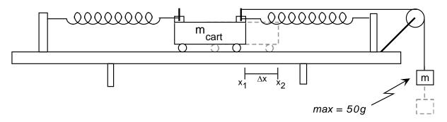
5. With the springs attached to the cart, record the equilibrium position of one end of the cart,  $x_1$  (the cart should be at rest).
