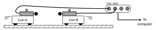
Securely fastened the force sensors on the carts. The rubber tips should be *carefully aligned* so that they will collide head-on with each other. Be sure that the switch on the force sensors is set to  $\pm 50$ N.
