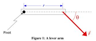
Notice that a longer lever arm results in a larger torque. A larger force also results in a larger torque, as well as a value of  $\theta$  closer to 90°. A torque can cause an object to rotate in a clockwise or counterclockwise fashion. A clockwise rotation is denoted as a negative torque; a counter-clockwise rotation is denoted by a positive torque. For an object to be in equilibrium, the sum of the torques acting on an object must equal zero.
