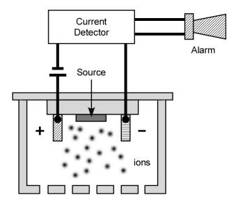
There are two types of smoke detectors available to consumers. One kind indicates the presence of smoke when it interferes with a photoelectric beam of light in the detector. The smoke detectors we will examine in this experiment are ionization-type detectors.
