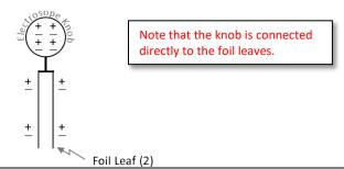
b. Charge the rubber rod with a piece of fur and bring it close to the knob of the (neutral) electroscope. On the sketch at right, draw (i) the leaves and an arrow showing how they have moved; (ii) the net charge on the rod (iii) charges on the knob and leaves. Be consistent with the total number of charges and *their expected position*. Briefly explain what happens to each foil leaf.
