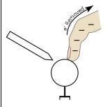
d. **First**, remove your finger, keeping the rod nearby. **Second**, remove the rubber rod. Draw leaves and charges on the sketch of the knob at the far right.
