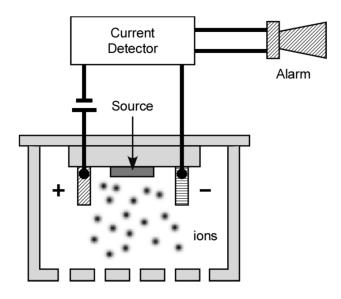
Appendix: How an Ionization-Type Smoke Detector Works<sup>1</sup>
