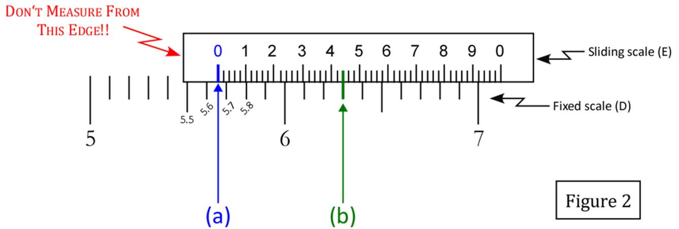
The measurement up to the first digit after the decimal point is obtained by looking at the line below the *first* zero (drawn thicker in *Figure 2* above for emphasis) that appears on the sliding scale (**E**), as indicated by point **(a)** above. In this example you will note that this line falls between the 5.6 and 5.7 cm line on the fixed scale (**D**), so we know our measurement falls within this range. Therefore, we'll start our measurement with **5.6**.
